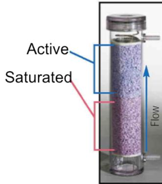
**Fig. 3.** Tube showing the difference between active (blue) saturated (pink) drierite. This chemical is anhydrous 97% calcium sulfate ( $\text{CaSO}_4$ ) and 3% cobalt chloride, and absorbs 6.6% its weight of water. When drierite changes to pink after water absorption, it should be replaced.
